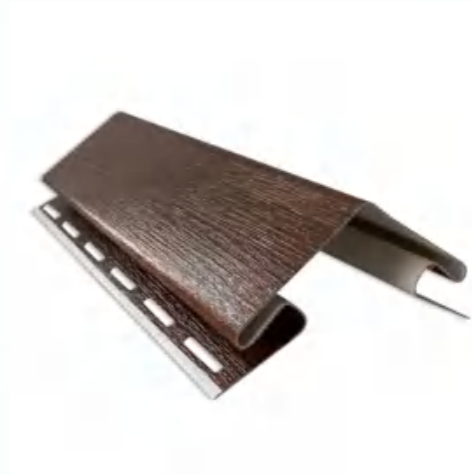
Name: Exterior Angle Column Length: 3.81m (150") Thickness: 0.9mm (0.035") Wight: 0.504 (±0.1kg) kgs/m
